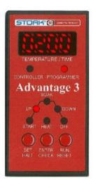
Continue this procedure to enter new values for **UP** rate, **SOAK** temperature, **SOAK** time, **DOWN** rate and **OFF** temperature.
