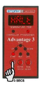
To end the HALT function press the HALT button once.
