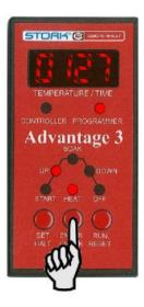
For a Controller Unit press and hold the **CHECK** button. The set point value is displayed until the button is released.
