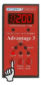
The value is changed one digit at a time by pressing the **SET** button to increment a digit . . . .
