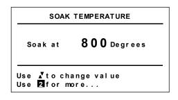
Press button 2 to return to **Profiler Overview** display. If no buttons are pressed for 20 seconds then the display will revert back to the **Profiler Overview**
