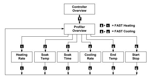
The user moves between each display by pressing one of the buttons. The instrument will emit a short beep every time a button is pressed.
