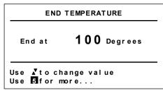
Press button 5 to return to **Profiler Overview** display. If no buttons are pressed for 20 seconds then the display will revert back to the **Profiler Overview**.
