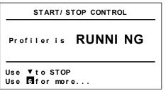
If the profiler is ready (not running) then press the up button to start the profile.
