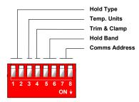
Switches 1 and 2 are used to select the type of hold operation.
