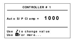
If no buttons are pressed for 20 seconds then the display will automatically revert back to the **Controller Overview**.
