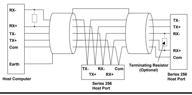
The above diagram shows the connections for 4 wire RS422 operation. This method of connection uses a separate pair of wires for transmission and reception and is the preferred connection method. Although called the '4 wire' connection, a fifth common wire is shown on the diagram. This wire should be fitted if at all possible
