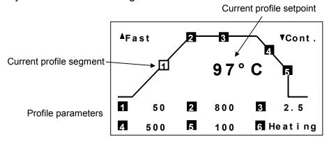
The diagram shows a typical heat-soak-cool profile with each stage numbered. The large number in the centre of the display shows the current profile setpoint with the current segment indicated by a flashing number.
