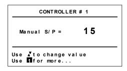
If no buttons are pressed for 20 seconds then the display will revert back to the **Controller Overview**.
