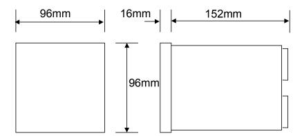
The instrument projects behind the panel by less than 152mm including terminal connections If IP65 sealing is required then ensure that the panel sealing gasket is fitted into position behind the bezel. The gasket may be omitted If IP65 sealing is not required.
