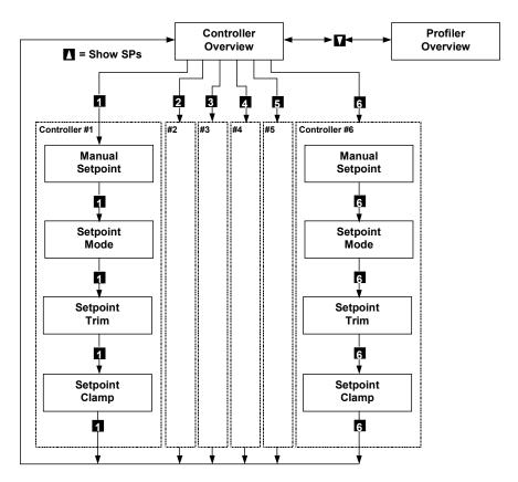
The user moves between each display by pressing one of the buttons. The instrument will emit a short beep every time a button is pressed.
