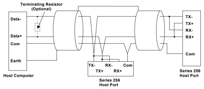
The above diagram shows the connections for 2 wire RS485 operation. This method of connection uses a single pair of wires for both transmission and reception with the data direction being controlled by the currently active device. As in the 4 wire connection, a common wire is shown on the diagram. This wire should be fitted if at all possible.
