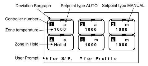
Each zone controller is represented by a rectangle on the display. Within this rectangle the current zone temperature is shown along with the setpoint mode.
