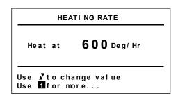
Press button 1 to return to **Profiler Overview** display. If no buttons are pressed for 20 seconds then the display will revert back to the **Profiler Overview**.
