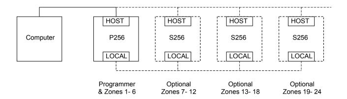
The serial communications may be connected using either the two or four wire system. The instrument uses a balanced voltage communications system which will perform well under most situations provided some simple guidelines are observed.
