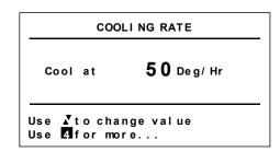
Press button 4 to return to **Profiler Overview** display. If no buttons are pressed for 20 seconds then the display will revert back to the **Profiler Overview**.
