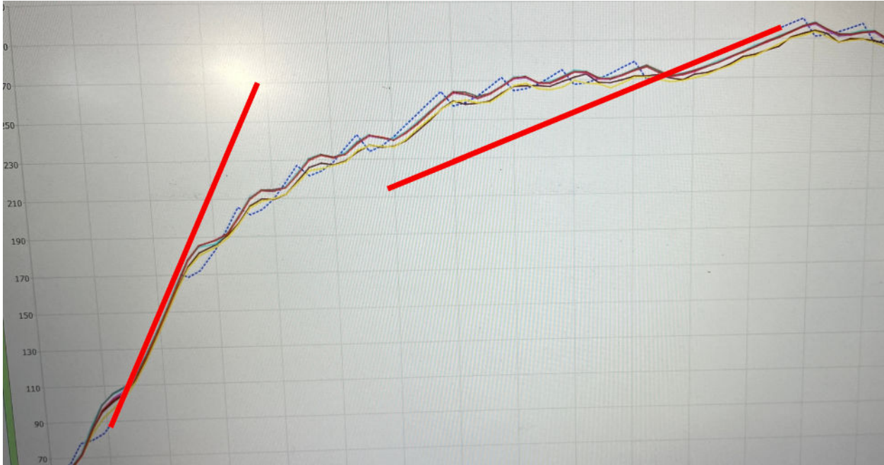
Figure 61: highlighting the difference in ramp rate after the system kept automatically adjusting the ramp rate because the system did not have enough power to heat at the desired rate.
