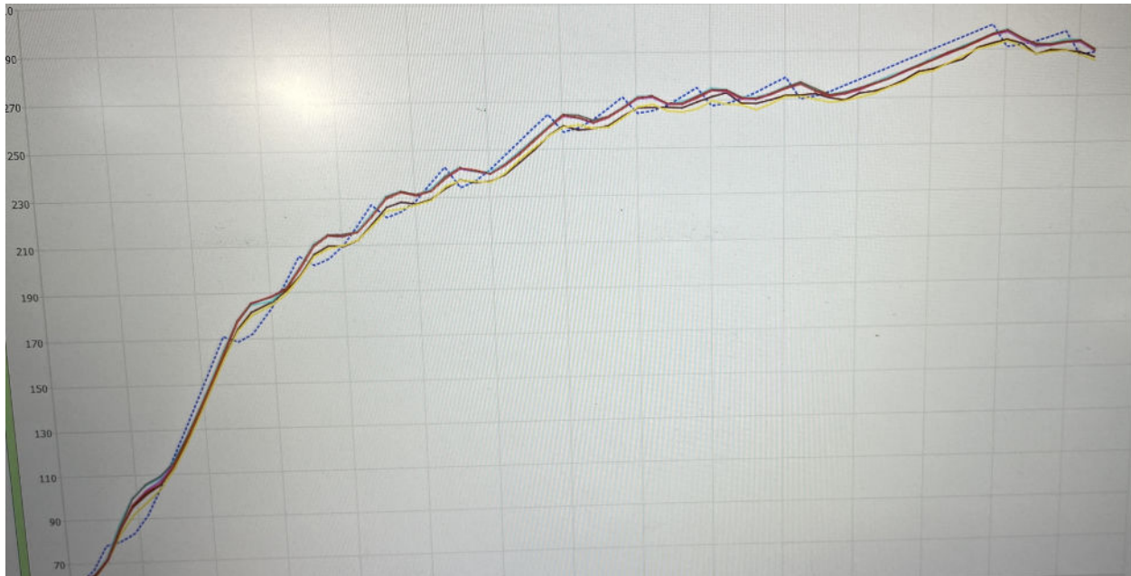
Figure 60: The system adjusting the ramp rate during a cycle as the system did not have enough power to heat the workpiece as fast as the operator desired
