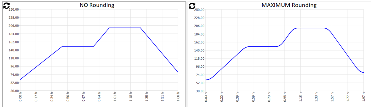
Figure 50: The difference in corner rounding.
