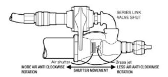
4.8 Turn on gas supply and light first burner using push button spark igniter. If damaged or missing light on - front face with a match.
