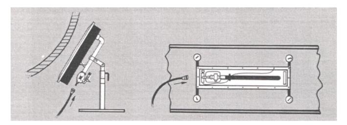
4.5 Connect gas supply hose to an isolated gas supply (i.e. propane bottle/network or natural gas supply).
